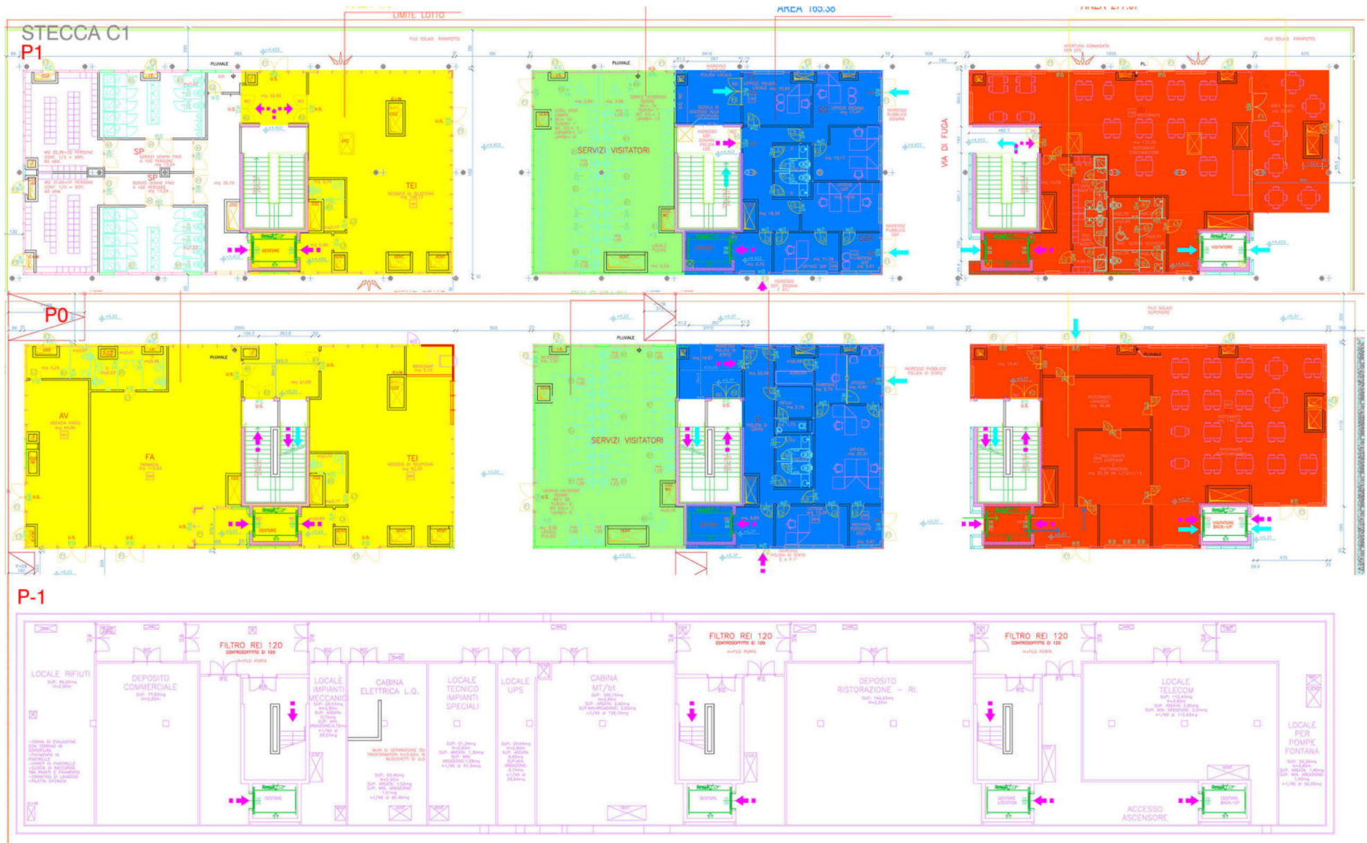
A map illustrating the gross zones dedicated for restaurants, commercial activities and spaces for police and sanitary services
